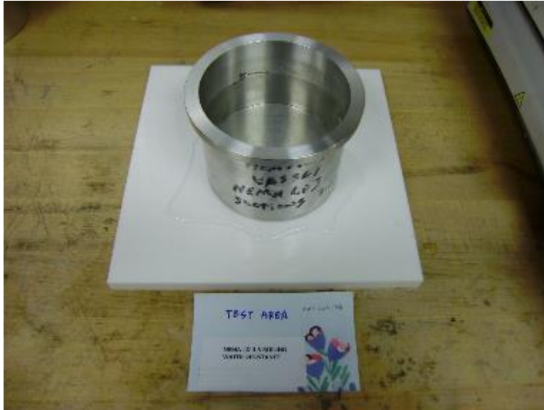
Photo No. 3 NEMA LD 3.5 Boiling Water Resistance Specimen with Heating Vessel Placed on 10 ml of Water
