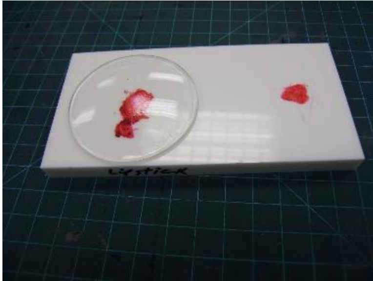
Photo No. 19 ANSI Z124.3 Sec. 5.2 Stain Resistance Test Lipstick Pre-Test
