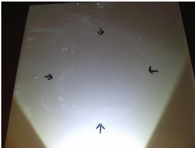
Photo No. 4 NEMA LD 3.6 High Temperature Resistance Evaluation of the Hot Wax Method - Test Result
