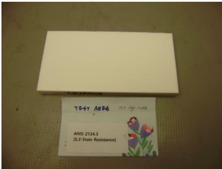
Photo No. 20 ANSI Z124.3 Sec. 5.2 Stain Resistance Test Lipstick Post-Test After Cleaning
